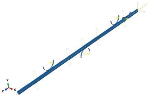
Figure 8: Whole model to simulate drawing, tensile and bending tests.
